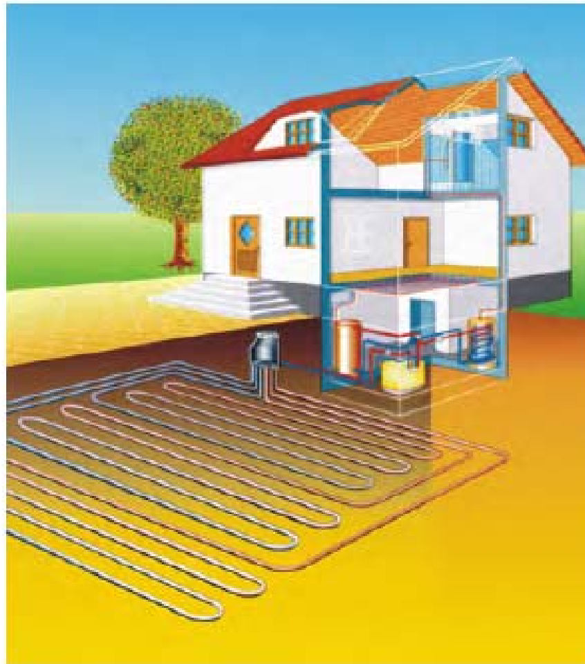
Fig. 8.28 Horizontal Earth coupled heat exchanger system (after [1999Ano a ]; yellow box in building basement: heat pump).
